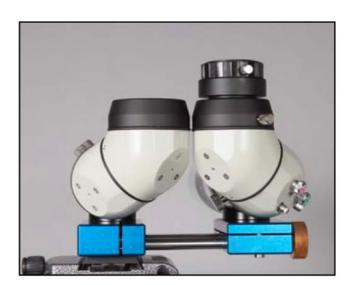
Also make sure that the two quickadjustment screws on the right-hand deflection system are in a central position so that they can be turned equally in both directions.
