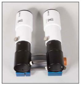
After you have screwed the two telescopic tubes onto the adjustment platform, you can attach the two Matsumoto deflecting mirror systems to the two tubes. Make sure that the two upper connection rings are as exactly parallel to the platform blocks as possible.
