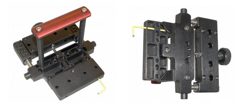
There are two M4 screws for this adjustment. Use a suitable Allen key as shown.
