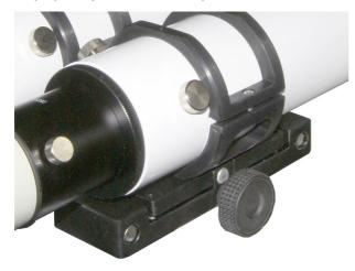
Look with both eyes through the two eyepieces and pay attention at the present moment only to a pleasant, overlapping image. The two telescopes will probably not be looking in the same direction. It is best not to focus at all before adjusting the telescope, but only to ensure a comfortable viewing experience.
