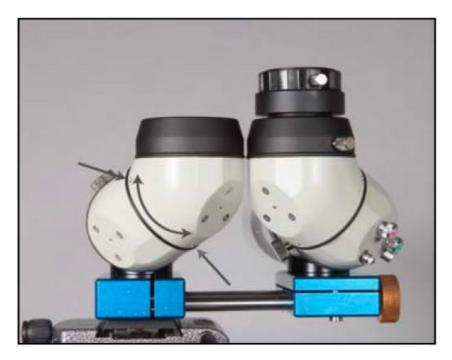
When observing with rather long focal length wide angle eyepieces, you will notice that the image - if congruent - is not equally centred in the two eyepieces. This is an effect of the interaction of your own eyes and the large viewing angles. If you use high magnification eyepieces with a rather narrow field of view, the image will tend to match.
