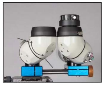
Mount the two telescopic tubes on the two platform blocks as parallel as possible by eye. Make sure that the tubes are really screwed tight.
