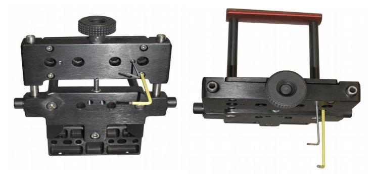
You now have a set of tension and compression bolts on the bottom of the right telescopic platform. This platform also has an axle in the middle.
