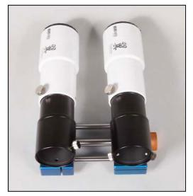
After vou have screwed the two telescopic tubes onto the adjustment platform. attach the you can two Matsumoto deflecting mirror systems to the two tubes. Make sure that the two upper connection rings are as exactly parallel to the platform blocks as possible.
